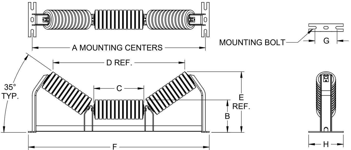
CEMA C 35° IMPACT TROUGHING IDLER 4" DIAMETER ROLLS
